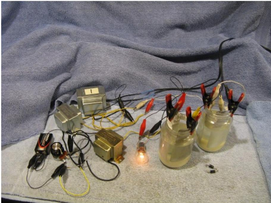
I was curious to see if homemade borax rectifiers (in the two jars) could be used instead of modern silicon rectifiers to increase the gain of the mag amp circuit. The answer is: They can indeed.
